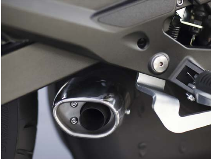
Midship muffler looks trick and aids mass centralisation
